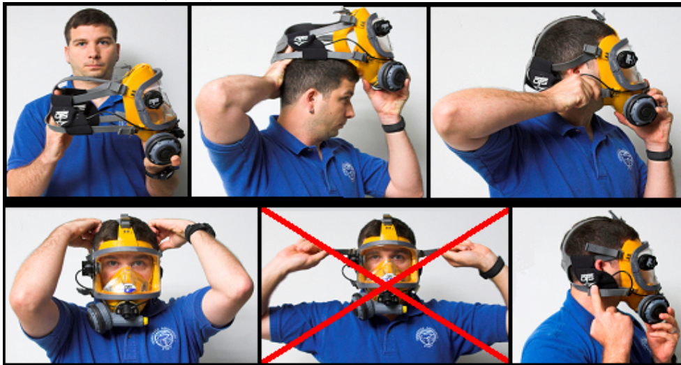
Figure 9 – Proper donning technique for the Divator MK II. Never pull the straps away from the head. The bone phone should be positioned just behind the ear.
